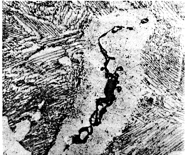
Figure 3. Fissure in 1095 vacuum steel after exposure to hydrogen for 3 hours at 10,000 psig and 930 F. 1000X etched 1% Nital.
